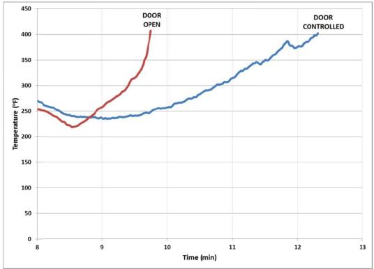
Figure 4.3: One-Story Living Room Temperatures after Front Door Open and Before Roof Open
