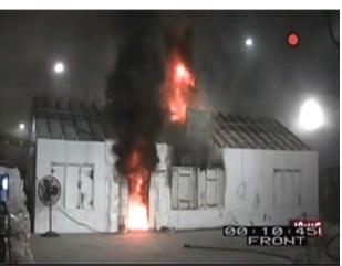
Figure 4.5: 5 seconds after roof vent
