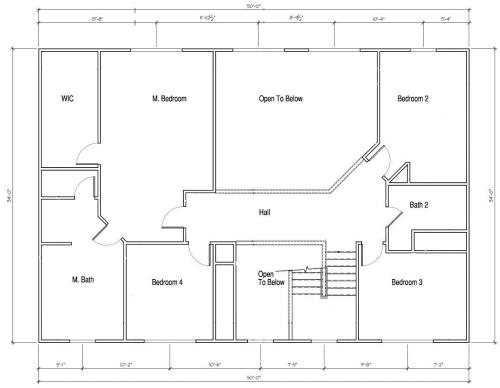
Figure 3.12. Two-Story House Second Floor Plan
