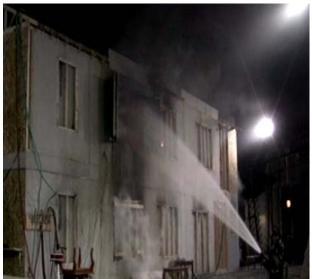
Figure 4.36: Fog Stream Sealing Flow Path
