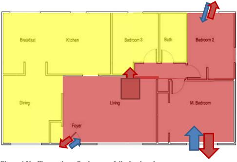
Figure 4.20: Flow paths as fire becomes fully developed
