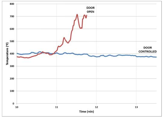
Figure 4.4: Two-Story Family Room Temperatures after Front Door Open and Before Roof Open
