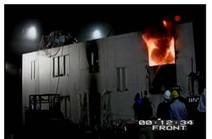
Figure 4.28: Water being applied from outside the house
