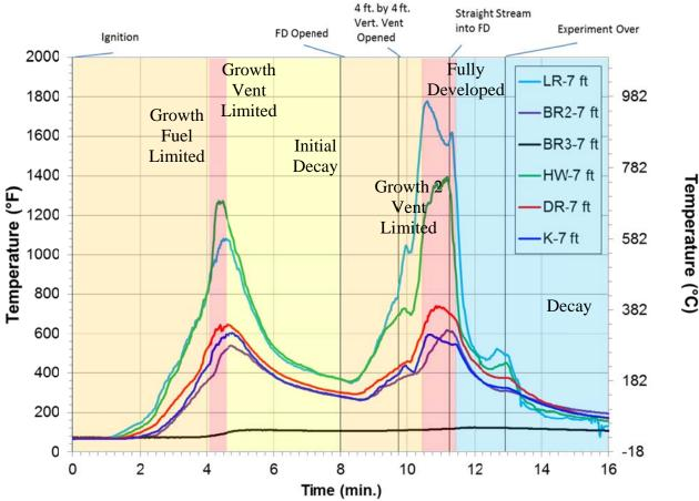
Figure 4.13: Experiment 5 Stages of Fire Development
