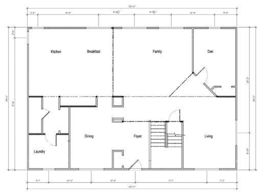
Figure 3.11. Two-Story House First Floor Plan
