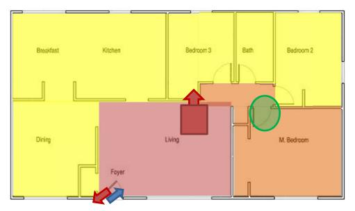
Figure 4.17: Flow path after the living room reaches flashover
